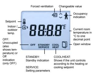
It is possible to set different parameter values in a parameter menu in the display, using the buttons on the controller. You change parameter values with the INCREASE and DECREASE buttons and confirm changes with the Occupancy button.
