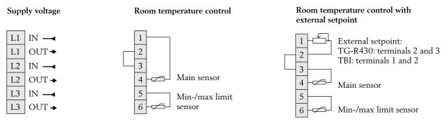
NOTE: When controlling Y-connected loads, the load must be symmetric and the signal neutral must not be connected!
