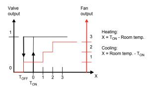
When there is no heating or cooling demand in the Auto position, the fan will run at the lowest speed. This can be changed in parameter 31 so that the fan stops when there is no heating or cooling demand. The fan is inactive in the Off and Window modes. However, it will continue to run if mould protection has been configured.
